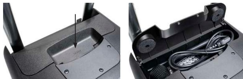
**EN** The accessory compartment provides space for up to two handheld transmitters, receiver antennae, remote control, power cord and other accessories. Pressing on the highlighted area (PUSH) opens up the cover (see figure). To close the cover, proceed in the same way.
